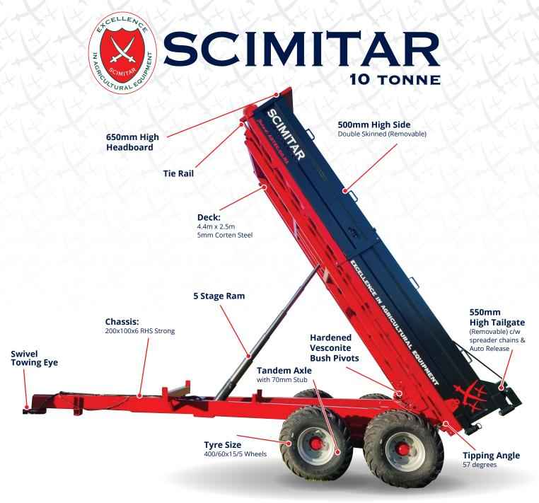
SCIMITAR 10 Tonne Tip Trailer built here in NZ and is designed to endure & survive the most intense conditions this trailer is put to. With over 30 years of experience in the farming sector and manufacturing we have come up with this strong and robust tip trailer, with heavy duty long lasting pivots, swivel towing eye, 5mm Corten steel deck and a strong chassis to ensure its capable of going beyond its expectations.
