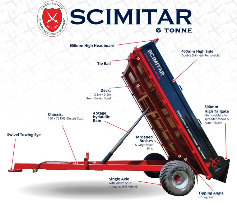
SCIMITAR 6 Tonne Tip Trailer built here in NZ and is designed to endure & survive the most intense conditions this trailer is put to. With over 30 years of experience in the farming sector and manufacturing we have come up with this strong and robust tip trailer, with heavy duty long lasting pivots, swivel towing eye, 4mm Corten steel deck and a strong chassis to ensure its capable of going beyond its expectations.
